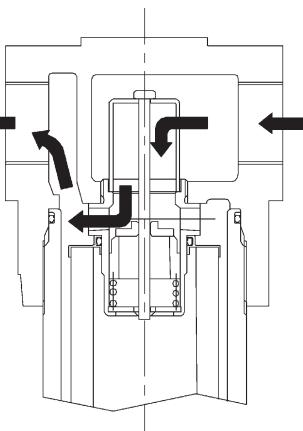
For hydraulic systems where reverse flow can occur, the pressure filters series FPB2+ and FPB3+ are available with a free reverse flow valve allowing the fluid to pass through the filter element in the normal direction and to bypass the filter element in the reverse direction (option "R"). The reverse flow valve is available also with incorporated bypass valve for the normal flow direction, set at 6 bar (option "P").
