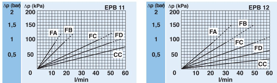
**CLEAN FILTER ELEMENT PRESSURE DROP WITH F+ AND C+MEDIA**
